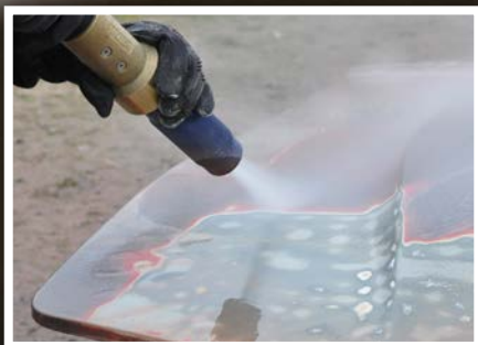
Coating and Paint Removal
