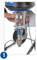
Remove rod coupling, inlet hose and paint
