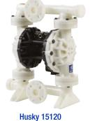
1-1/2 in (38.1 mm) connection Max flow: 454 lpm (120 gpm) Polypropylene, PVDF
