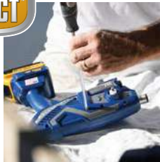
1. Remove the cover with a screwdriver.
