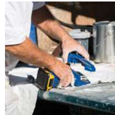
2. Remove the old pump from the sprayer.
