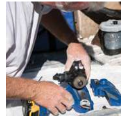
3. Place the new pump into sprayer.
